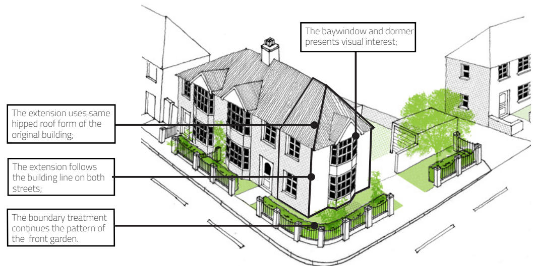
An example of corner plot side extension with design features respect its surrounding environment.
