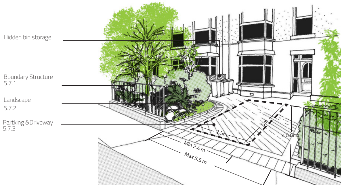
An example implementing the guidelines for creating a new drive way in front garden
